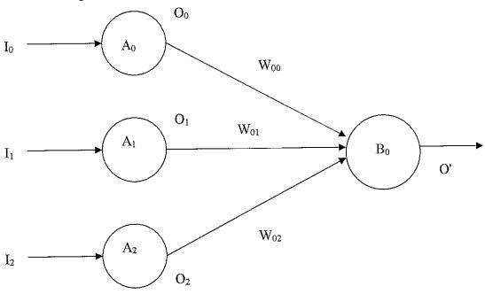
The input layer neurons simply copy their input to the output, i.e.  $O_i = I_i$ , i = 0, 1, 2. The output neuron works using the weights  $W_{00}$ ,  $W_{01}$ ,  $W_{02}$ , and the sigmoidal function f, the details of which are given below.
