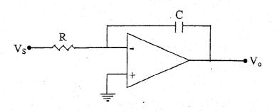
4) The circuit shown uses an op-amp, that is ideal, except for having a finite gain A. Measurements indicate  $V_0 = 3.5V$ . When  $V_1 = 3.5V$ , what is the op-amp gain A? [3 marks]
