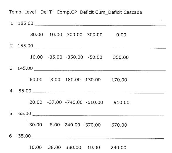
2. For the heat exchanger network synthesis problem given below, hot and cold utility requirements for HRAT = 8 °C are 4800 kW each. The pinch temperature is 104 °C.
