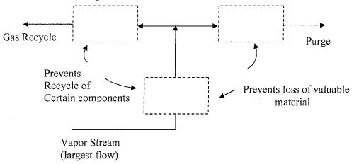
**Location of a vapor-recovery system**: There are four choices for the location of the vapor-recovery system:
