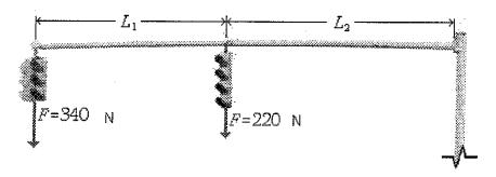
L1= L2= 250cm. Radius of the cylindrical solid rod = 4cm. E=200GPa. [8 Marks]
