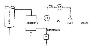
4) Consider the Cascade control system shown in Figure below:
