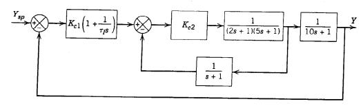
a) Specify K<sub>c2</sub>, so that the gain margin > 1.7 and phase margin > 30° for the slave loop (2.5 Marks)
