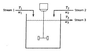
Derive a dynamic model that will describe transient operation. Make a degree of freedom analysis assuming that both stream1 and 2 come from upstream units (i.e their flow rates and temperature are known function of time) (2+1=3.0 M)
