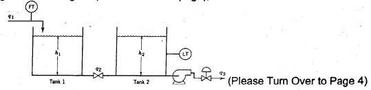
(A)the two tanks have uniform cross sectional areas,  $A_1$  and  $A_2$ , respectively. (B)the valve on the exit line of Tank 1 acts as a linear resistance with a flow-head relation,  $q_2=(h_1-h_2)/R$ . (C)The transmitters and control valve are pneumatic instruments that have negligible dynamics. (D)The pump operates so that flow rate  $q_3$  is independent of  $h_2$  when the control valve stem position is maintained constant.
