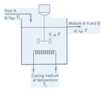
6) A stirred tank blending system initially is full of water and is being fed pure water at a constant flow rate,  $q = 0.4 \text{ m}^3/\text{min}$ . At a particular time (say, t=t<sub>1</sub>), an operator adds caustic solution of concentration <u>c</u><sub>i</sub> at the same volumetric flow rate q. If the liquid volume
