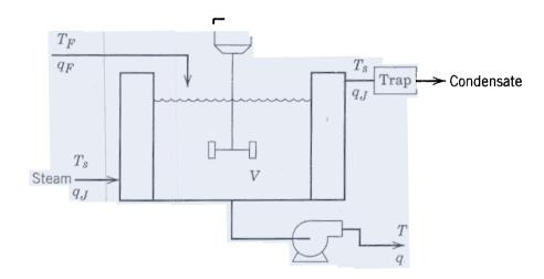
Derive a dynamic model for this process by determining different transfer functions relating the two primary output variables h (level) and T(liquid temperature) to inputs  $q_F$ , q and  $T_s$ . Note:-The model should be simplified as much as possible. State any additional assumptions that you make. (6.0 M)
