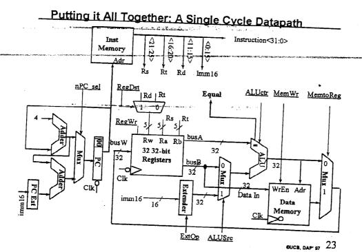
for one input of ALU data may come from busB or 16-bit sign extended to 32 bit depending on Add instruction or LW instruction. To resolve this appropriate multiplexer is needed. For addressing the registers one multiplexer is needed because Rd field will decide the destination register in case of Add instruction-whereas in some instructions like logical operations Rt will decide the destination. Similar reasons should be given to other multiplexers also (1 +5) marks
