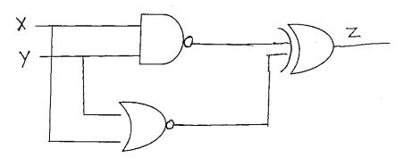
2b) In the logic circuit given below, find the redundant gate, by using K'MAP
