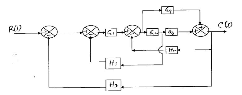
3. Derive the Transfer Function of the figure of question 2 using Signal Flow Graph and Mason's Gain formula. [8]
