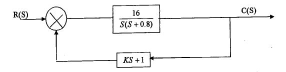
10. The open loop transfer function of a unity feedback system is given below. Sketch the Polar plot
