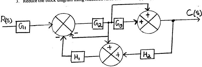
4. Find the overall Transfer Function of the following system using Mason's Gain Formula.
