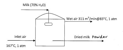
Calculate the production rate of dried milk and the volumetric flow rate of the inlet air. Estimate upward velocity of air (m/min) at the bottom of the dryer.
