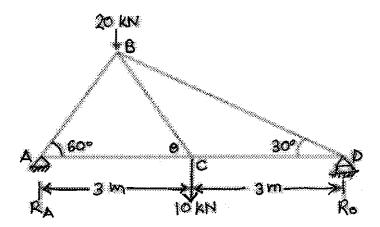
**Q4.** A small railroad bridge is constructed with steel members, all of which have a cross-sectional area of 3250 mm<sup>2</sup>. A strain stops on the bridge and the loads applied to the truss on one side of the bridge are shown in the sketch. Estimate how much the point R moves horizontally because of this loading. [10M]
