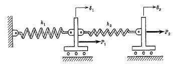
Q4.Draw the force vs deflection graph for work done and complementary work done for a force F acting on a spring mass system which produces a deflection  $\delta$ . [1 M]
