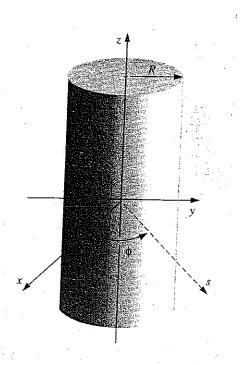
4. A coaxial cable consists of two very long cylindrical tubes, separated by linear insulating material of magnetic susceptibility  $\chi_m$ . A current I flows down the inner conductor and returns along the outer one, in each case the current distributes itself uniformly over the surface. Find the magnetic field in the region between the tubes and also calculate the bound currents . (6M)
