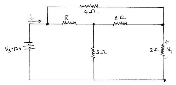
Q2. Consider the following circuit and determine the values of v,  $i_1$  and  $i_2$ . [5M]
