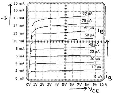
2. A transistor has a  $\beta$  of 250 and a base current,  $\dot{\boldsymbol{\zeta}}_B$ , of 20  $\mu$  A. The collector current,  $\dot{\boldsymbol{\zeta}}_C$ , equals \_\_\_\_ [1 M]
