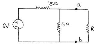
6. Draw the Norton's equivalent to the left of a and b for the Thevenin's circuit shown below.
